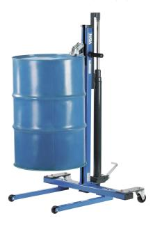
for pick up and transport of 200 l-drums, user friendly pump with food lever, safe and exact kneeling possible, the legs are adapted to euro pallets. Painted blue RAL 5010. Dimensions approx.: Frame width outside: 960 mm Frame width inside: 870 mm Height min./max.: 1410/1915 mm Length complete: 850 mm Length of legs: 570 mm Height of legs: 65 mm 2 stand rollers with dia = 65 mm 2 slewable with dia = 80 mm Lift height: 700 mm Load bearing capacity: 300 kg Weight: 67 kg
