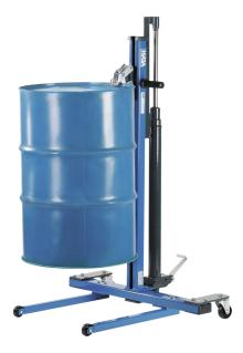
for pick up and transport of 200 l-drums, user friendly pump with food lever, safe and exact kneeling possible, the legs are adapted to euro pallets. Painted blue RAL 5010. Dimensions approx.: Frame width outside: 960 mm Frame width inside: 870 mm Height min./max.: 1410/1915 mm Length complete: 850 mm Length of legs: 570 mm Height of legs: 65 mm 2 stand rollers with dia = 65 mm 2 slewable with dia = 80 mm Lift height: 700 mm Load bearing capacity: 300 kg Weight: 67 kg
