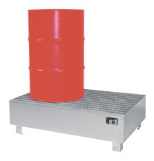
dimensions:approx.  $1200 \times 800 \times 360 \text{ mm}$  (L x W x H) collection volume: 215 I material strength 3 mm, with galvanised removable gratings with supporting feet, 100 mm underclearance suitable for flammable liquids F+, F and water polluting liquids WGK 1 - 3 Testings: with declaration of conformity (ÜHP) according to StawaR Tested by TÜV
