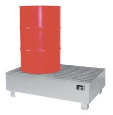
dimensions:approx. 1200 x 800 x 360 mm (L x W x H) collection volume: 215 l material strength 3 mm, with galvanised removable gratings with supporting feet, 100 mm underclearance suitable for flammable liquids F+, F and water polluting liquids WGK 1 - 3 Testings: with declaration of conformity (ÜHP) according to StawaR Tested by TÜV
