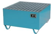
Dimensions: approx. 800 x 800 x 465 (WxDxH in mm) Collection volume: 210 I Colour RAL 5012 blue, material strength 3 mm, with galvanised removable grating, skids with 100 mm underclearance, Load: 250 kg Suitable for flammable liquids F+, F und for water polluting liquids WGK 1-3 Testings: Declaration of conformity (ÜHP) according to StawaR, TÜV-tested
