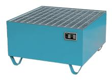
Dimensions: approx. 800 x 800 x 465 (WxDxH in mm) Collection volume: 210 l Colour RAL 5012 blue, material strength 3 mm, with galvanised removable grating, skids with 100 mm underclearance, Load: 250 kg Suitable for flammable liquids F+, F und for water polluting liquids WGK 1-3 Testings: Declaration of conformity (ÜHP) according to StawaR, TÜV-tested
