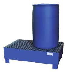
Approx. dim.: 1200 x 800 x 360 (WxDxH in mm) Collection volume: 200 l Colour RAL 5010 blue, material strength 3 mm, with galvanised removable grating, skids with 100 mm underclearance, Load: 500 kg Suitable for flammable liquids F+, F und for water polluting liquids WGK 1-3 Testings: Declaration of conformity (ÜHP) according to StawaR,
