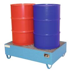
Approx. dim.: 1200 x 800 x 360 (WxDxH in mm) Collection volume: 200 l Colour RAL 5012 blue, material strength 3 mm, with galvanised removable grating, skids with 100 mm underclearance, Load: 500 kg Suitable for flammable liquids F+, F und for water polluting liquids WGK 1-3 Testings: Declaration of conformity (ÜHP) according to StawaR, TÜV-tested
