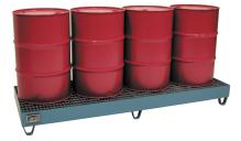
Dimensions: appr. 2400 x 800 x 250 (WxDxH in mm) Collection volume: 210 l Colour RAL 5012 blue, material strength 3 mm, with galvanised removable grating, skids with 100 mm underclearance, Load: 1000 kg Suitable for flammable liquids F+, F und for water polluting liquids WGK 1-3 Testings: Declaration of conformity (ÜHP) according to StawaR, TÜV-tested
