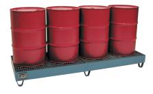
Dimensions: appr. 2400 x 800 x 250 (WxDxH in mm) Collection volume: 210 l Colour RAL 5012 blue, material strength 3 mm, with galvanised removable grating, skids with 100 mm underclearance, Load: 1000 kg Suitable for flammable liquids F+, F und for water polluting liquids WGK 1-3 Testings: Declaration of conformity (ÜHP) according to StawaR, TÜV-tested
