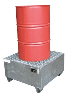
Approx. dim.: 800 x 800 x 465 (WxDxH in mm) Collection volume: 210 I Material strength 3 mm, with galvanised removable grating, skids with 100 mm underclearance, Load: 250 kg Suitable for flammable liquids F+, F und for water polluting liquids WGK 1-3 Testings: Declaration of conformity (ÜHP) according to StawaR, TÜV-tested
