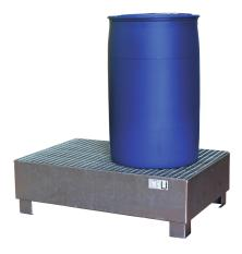
Approx. dim.:  $1200 \times 800 \times 360$  (WxDxH in mm) Collection volume: 210 I Material strength 3 mm, with galvanised removable grating, skids with 100 mm underclearance, Load: 500 kg Suitable for flammable liquids F+, F und for water polluting liquids WGK 1-3 Testings: Declaration of conformity (ÜHP) according to StawaR
