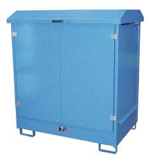
painted with 2 wings doors for 2 drum 200 litre Dims.:  $1437 \times 1015 \times 1614$  mm (L x W x H) Collection vol.: 210 l painted external surface blue RAL 5012 with natural air exchange collection tray with galvanised graiting Roof with pneumatic springs, lockable fork stirrups with 100 mm underclearance for flammable liquids F+, F and water polluting liquids in water pollution class WGK 1-3. Testing: With general national technical approval Z-38.5-101 (DIBt Berlin), TÜV-tested
