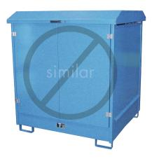
painted with 2 wings doors for 4 drum 200 litre Dims.:  $1437 \times 1500 \times 1557 \text{ mm}$  (L x W x H) Collection vol.: 220 l painted external surface blue RAL 5012 with natural air exchange collection tray with galvanised graiting Roof with pneumatic springs, lockable fork stirrups with 100 mm underclearance for flammable liquids F+, F and water polluting liquids in water pollution class WGK 1-3. Testing: With general national technical approval Z-38.5-101 (DIBt Berlin), TÜV-tested
