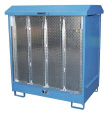
painted with 2 wings doors for 2 drum 200 litre Dims.: 1437 x 1015 x 1514 mm (L x W x H) Collection vol.: 210 I painted external surface blue RAL 5012 with natural air exchange collection tray with galvanised graiting Roof with pneumatic springs, lockable with fold down front door made from aluminium as ramp, for flammable liquids F+, F and water polluting liquids in water pollution class WGK 1-3. Testing: With general national technical approval Z-38.5-101 (DIBt Berlin), TÜVtested
