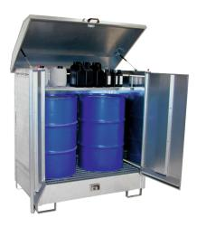
galvanised with 2 wings doors for 2 x 200 l-drums Dims.:  $1437 \times 1015 \times 1614 \text{ mm}$  (L x W x H) Collection vol.: 210 l painted external surface blue RAL 5012 with natural air exchange collection tray with galvanised grating Roof with pneumatic springs, lockable fork stirrups with 100 mm underclearance for flammable liquids F+, F and water polluting liquids in water pollution class WGK 1-3. Testing: With general national technical approval Z-38.5-101 (DIBt Berlin), TÜV-tested
