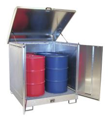
galvanised with 2 wings doors for 4 x 200 l-drums, Dims.:  $1437 \times 1500 \times 1557 \text{ mm}$  (L x W x H) Collection vol.: 220 l with natural air exchange collection tray with galvanised grating Roof with pneumatic springs, lockable fork stirrups with 100 mm underclearance for flammable liquids F+, F and water polluting liquids in water pollution class WGK 1-3. Testing: With general national technical approval Z-38.5-101 (DIBt Berlin), TÜV-tested
