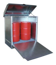
galvanised with ramp for 2 x 200 l-drums, Dims.:  $1437 \times 1015 \times 1514 \text{ mm}$  (L x W x H) Collection vol.: 210 l with natural air exchange collection tray with galvanised grating Roof with pneumatic springs, lockable with fold down front door made from aluminium as ramp, for flammable liquids F+, F and water polluting liquids in water pollution class WGK 1-3. Testing: With general national technical approval Z-38.5-101 (DIBt Berlin), TÜV-tested
