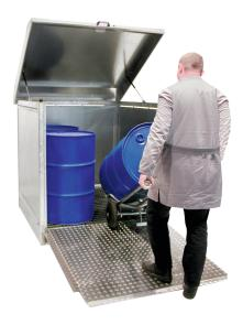
galvanised with ramp for 4 x 200 l-drums Dims.:  $1437 \times 1500 \times 1457 \text{ mm}$  (L x W x H) Collection vol.: 220 l with natural air exchange collection tray with galvanised grating Roof with pneumatic springs, lockable with fold down front door made from aluminium as ramp, for flammable liquids F+, F and water polluting liquids in water pollution class WGK 1-3. Testing: With general national technical approval Z-38.5-101 (DIBt Berlin), TÜV-tested
