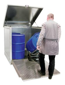
galvanised with ramp for 4 x 200 l-drums Dims.: 1437 x 1500 x 1457 mm (L x W x H) Collection vol.: 220 l with natural air exchange collection tray with galvanised grating Roof with pneumatic springs, lockable with fold down front door made from aluminium as ramp, for flammable liquids F+, F and water polluting liquids in water pollution class WGK 1-3. Testing: With general national technical approval Z-38.5-101 (DIBt Berlin), TÜV-tested
