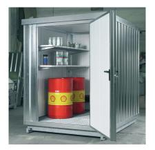
INSULATED, GALVANISED VERSION: Outer dim.: 1950 x 2350 x 2340(WxDxH in mm) Inner dim.: 1772 x 2062 x 2051 (WxDxH in mm) Capacity: 6300 l Approval for storage of water polluting liquids WGK 1 - 3, flammable liquids, F+, F outdoors or in building in accordance with the specific fire protection regulations. Construction of container:
