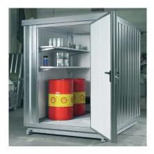
INSULATED, GALVANISED VERSION: Outer dim.:  $1950 \times 2350 \times 2340$ (WxDxH in mm) Inner dim.:  $1772 \times 2062 \times 2051$  (WxDxH in mm) Capacity: 6300 I Approval for storage of water polluting liquids WGK 1 - 3, flammable liquids, F +, F outdoors or in building in accordance with the specific fire protection regulations. Construction of container:
