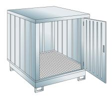
Sheet steel galvanized Outer dim.:  $1250 \times 1525 \times 1699$  (LxBxH in mm) Capacity: 2500 I Approval for storage of water polluting liquids WGK 1 - 3, flammable liquids, F+, F outdoors or in building in accordance with the specific fire protection regulations. Construction of container:
