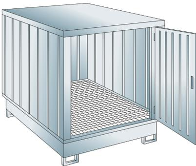
Sheet steel galvanized Outer dim.: 1550 x 1525 x 1669 (LxBxH in mm) Capacity: 2400 l Approval for storage of water polluting liquids WGK 1 - 3, flammable liquids, F+, F outdoors or in building in accordance with the specific fire protection regulations. Construction of container:
