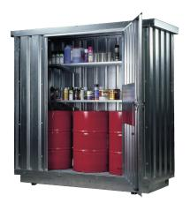
GALVANISED VERSION: Dimension: 915 x 2350 x 2340 (LxWxH in mm) Capacity: 3000 l Approval for storage of water polluting liquids WGK 1 - 3, flammable liquids, F+, F outdoors or in building in accordance with the specific fire protection regulations. Construction of container:
