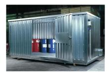
GALVANISED VERSION: Dimensions:  $2350 \times 5055 \times 2340$  (LxWxH in mm) Capacity: 10000 I Approval for storage of water polluting liquids WGK 1 - 3, flammable liquids, F+, F outdoors or in building in accordance with the specific fire protection regulations. Construction of container:
