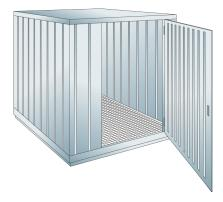
GALVANISED VERSION: Dimensions:  $1950 \times 2350 \times 2340$  (LxWXH in mm) Capacity: 6300 I Approval for storage of water polluting liquids WGK 1 - 3, flammable liquids, F+, F outdoors or in building in accordance with the specific fire protection regulations. Construction of container:
