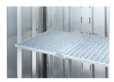
For safety storage containers. Dimensions: approx. 2000 x 500 (WxD in mm) consisting of: 2 shelving uprights 4 consoles (adjustable every 140 mm) 2 gratings Load bearing capacity per grating: 120 kg for for uniformly distributed load
