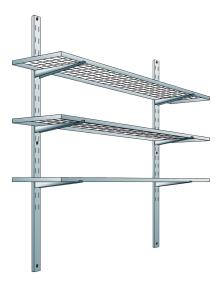
For safety storage containers. Dimension approx.:  $2000 \times 500$  (BxT in mm) consisting of: 2 shelving uprights 6 consoles (adjustable every 140 mm) 3 gratings Load bearing capacity per grating:  $120 \times 10^{-2}$  kg for uniformly distributed load
