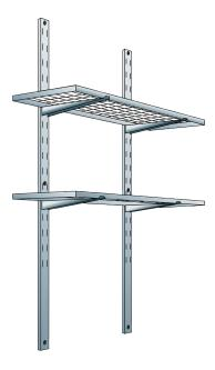
For safety storage containers. Dimension approx.:  $1000 \times 500$  (BxT in mm) consisting of: 2 shelving uprights 4 consoles (adjustable every 140 mm) 2 gratings Load bearing capacity per grating:  $120 \times 1000$  kg for uniformly distributed load
