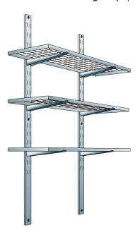
For safety storage containers. Dimension approx.:  $2000 \times 500$  (BxT in mm) consisting of: 2 shelving uprights 6 consols (adjustable every 140 mm) 3 gratings Load bearing capacity per grating: 120 kg for uniformly distributed load
