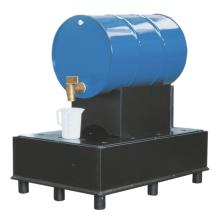
Dim.: appr. 1270 x 870 x 400 (W x D x H in mm), collection volume: 225 I load bearing capacity: 900 kg low tare weight: 62 kg plastic structure made from extruded laminate (PE-HD), with stable PE perforated plate as standing level accessiuble due to 100 mm base design. suitable for water polluting, non-flammable liquids WGK 1-3, Tested: General national technical approval of DIBT-Berlin, MPA-tested, TÜV-tested
