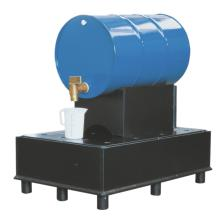
Dim.: appr.  $1270 \times 870 \times 400$  (W x D x H in mm), collection volume: 225 I load bearing capacity: 900 kg low tare weight:  $62 \text{ kg plastic structure made from extruded laminate (PE-HD), with stable PE perforated plate as standing level accessible due to <math>100 \text{ mm}$  base design. suitable for water polluting, non-flammable liquids WGK 1-3, Tested: General national technical approval of DIBT-Berlin, MPA-tested, TÜV-tested
