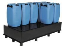
Dim.: appr. 1870 x 870 x 310 (W x D x H in mm), collection volume: 225 I load bearing capacity: 1350 kg low tare weight: 77 kg plastic structure made from extruded laminate (PE-HD), with stable PE perforated plate as standing level accessiuble due to 100 mm base design. suitable for water polluting, non-flammable liquids WGK 1-3, Tested: General national technical approval of DIBT-Berlin, MPA-tested, TÜV-tested
