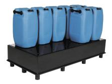
Dim.: appr. 1870 x 870 x 310 (W x D x H in mm), collection volume: 225 l load bearing capacity: 1350 kg low tare weight: 77 kg plastic structure made from extruded laminate (PE-HD), with stable PE perforated plate as standing level accessible due to 100 mm base design. suitable for water polluting, non-flammable liquids WGK 1-3, Tested: General national technical approval of DIBT-Berlin, MPA-tested, TÜV-tested
