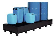
Dim.: appr. 2470 x 870 x 270 (W x D x H in mm), collection volume: 225 I load bearing capacity: 1800 kg low tare weight: 89 kg plastic structure made from extruded laminate (PE-HD), with stable PE perforated plate as standing level accessiuble due to 100 mm base design. suitable for water polluting, non-flammable liquids WGK 1-3, Tested: General national technical approval of DIBT-Berlin, MPA-tested, TÜV-tested
