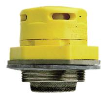
Of plastic and galvanised steel, 2" thread with flame arrester made from galvanised steel, automatic pressure compensation, automatic vacuum compensation for curved surface (belly) of drum
