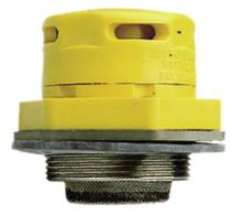
Of plastic and galvanised steel, 2" thread with flame arrester made from galvanised steel, automatic pressure compensation, automatic vacuum compensation for curved surface (belly) of drum
