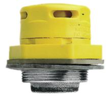
Of plastic and stainless steal, 2" thread with flame arrester made from stainless stell, automatic pressure compensation, automatic vacuum compensation for curved surface (belly) of drum
