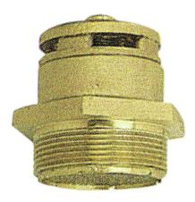
Of brass, 2"-thread, with flame arrester made from brass, automatic pressure compensation, automatic vacuum compensation for curved surface (belly) of drum
