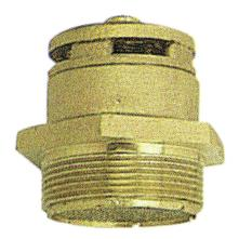
Of brass, 2"-thread, with flame arrester made from brass, automatic pressure compensation, automatic vacuum compensation for curved surface (belly) of drum
