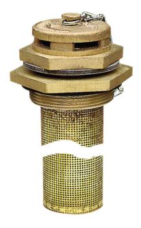
Of brass, 2"-thread, with flame arrester made from brass, 140 mm long, removable head, automatic pressure compensation, automatic vacuum compensation for curved surface (belly) of drum
