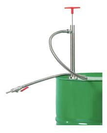
drum thread and non-return valve parts in contact with medium made from stainless steel 1.4301 and PTFE electro-statically conductive unscrewable outlet hose immersion depht: 910 mm delivery rate per stroke: 560 ml immersion depth: 1030 mm immersion tube dia: 32 mm
