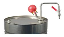
gaskets made from EPDM pump is gas-tight and can be completely blocked with two ball valves. immersion depth 600 mm suitable for stainlesss steel drums usually used in laboratories Flow rate: 10 l/min. with R 2 ''-fine thread
