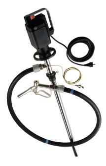
for highly flammable hydrocarbons drum pump set consisting of: drump pump, pump made from stainless steel 2 m solvent hose DN 25 conductive hose connections, equipotential bonding cable brass extracton nozzle and PP drum adapter degree of protection IP 54 230 V motor with 5 m cable, earthing pin plug explosion-proof in accordance with the Atex 100a guidelines electrical drive immersion depth: 1000 mm immersion tube Dia: 41 mm
