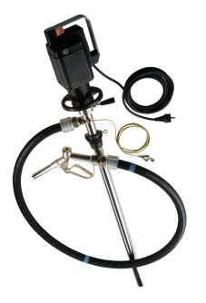
for highly flammable hydrocarbons drum pump set consisting of: stainless steel drum pump residue draining pump made from stainless steel, 2 m solvent hose DN 25 conductive hose connections, equipotential bonding cable brass extracton nozzle and PP drum adapter degree of protection IP 54 230 V motor with 5 m cable, earthing pin plug explosion-proof in accordance with the Atex 100a guidelines electrical drive immersion depth: 1000 mm immersion tube Dia: 41 mm
