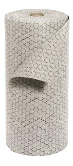
for industrial liquids non-woven fabric binders made from polyprophylene micro fibres , dimensions: approx 800 mm x 40 m lenghtwise perforation, every 500 mm, maximum absorption capacity per VE:  $162\ l$  We recommend to use the smooth surface which is sublimated with spin fleece as working document.
