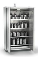
classical door technology (door handle), door hung right for the storage of flammable liquids. type testing by MPA/TÜV SÜD according to DIN EN 14470-1, DIN EN 16121 and DIN EN 16122, EK5/AK4 09-10:2009 and AfPS GS 2014: 01 PAK mark of approval: GS/CE mark, high quality mark of approval by TÜV SÜD construction and colour:
