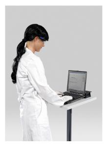
Analysing unit to log the tempertaures inside the refrigerators as well as the temperatures of the substances using the additional temperature probe, and to read out the refrigerator parameters such as compressor on/off, alarm states, etc.
