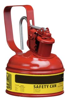
Dim.: 120 x 180 ( dia x H in mm ) interior tin plated exterior red powder coated Self-closing opening stainless steel flame arrester in can neck Automatic pressure compensation Marking prepared according to GefStoffV and BGV A8
